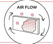
Keep items 1 ft away from the Radiator to ensure proper air intake to heat the room.
